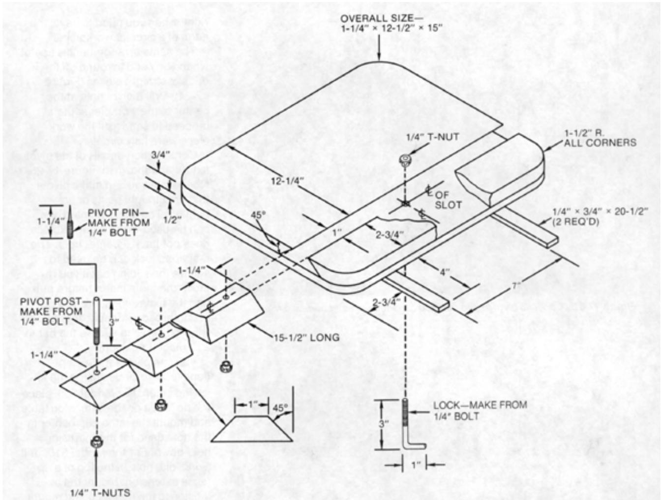
**Figure 17-25.** Construction details of the pivot fixture. Notice the two types of pivot posts; one has a point to be used when the workpiece does not have a center hole.
