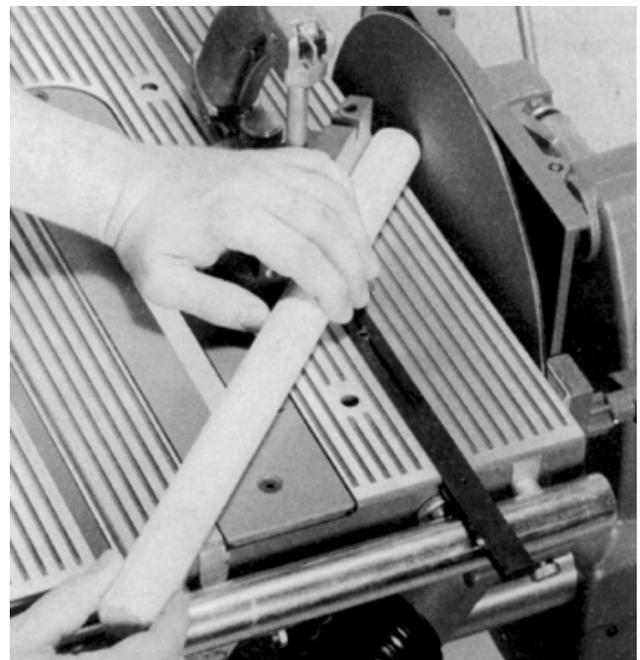
**Figure 17-29.** The ends of the dowels are larger rounds can be pointed or chamfered freehand by angling the miter gauge.
