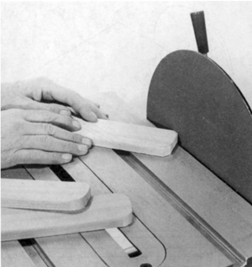
**Figure 17-27.** Corners can be rounded off by sanding to a line. The bulk of the waste should be removed with saw cuts before you begin.
