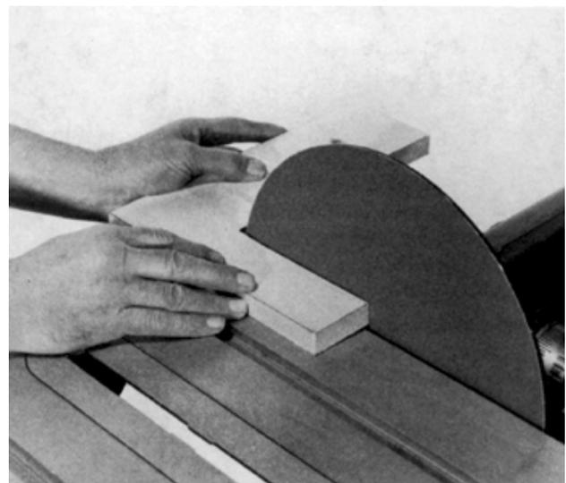
**Figure 17-10.** The second pass can be across the disc or directly into it, depending on the length of the work. The corner will require a bit of hand finishing.
