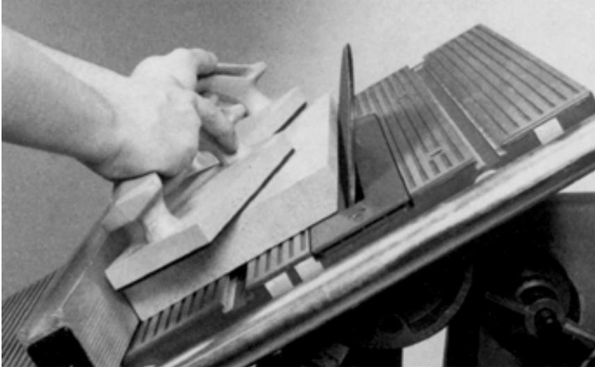
**Figure 17-17.** To sand a chamfer in the edge of a board, tilt the worktable and proceed as you would when edge sanding. Don't take off too much stock in one pass.
