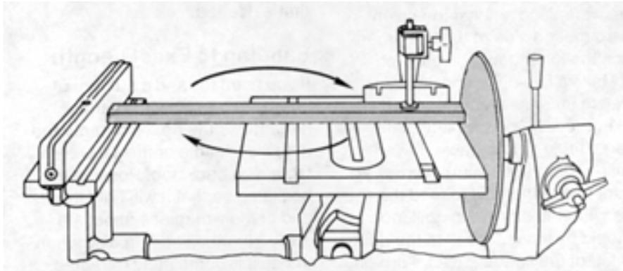
**Figure 17-6.** Sand one end of the board until it's smooth; then turn the board as shown and sand the other end until the depth control stops and sanding disc.
