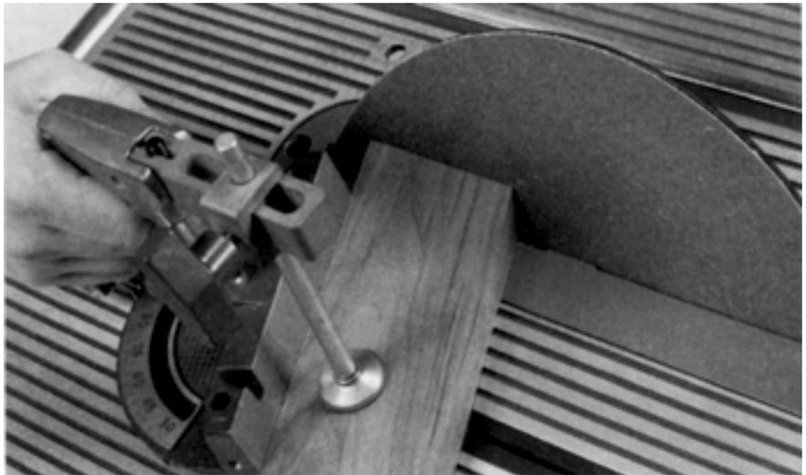
**Figure 17-15.** When sanding compound miters, keep the miter gauge and the worktable tilt at the same angles used when making the saw cut.
