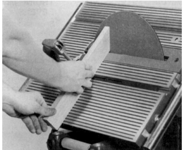
**Figure 17-12.** When sanding angles on the Model 510, position the sanding disc through the table saw insert.
