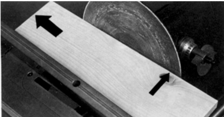
**Figure 17-16.** Boards can be sanded to width using this setup. In this case the worktable is tilted to sand a bevel. The large arrow indicates feed direction; the small one indicates the gap needed between the workpiece and the "rear" half of the disc.
