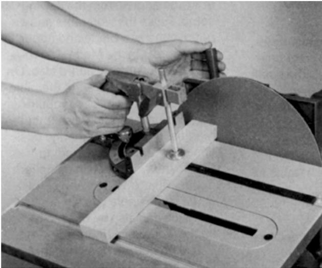
**Figure 17-11.** When sanding angles on the Model 500 use the quill to move the disc toward the stock.
