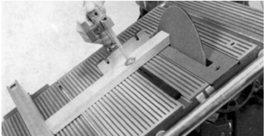
**Figure 17-14.** The rip fence can also be used to back up the workpiece.
