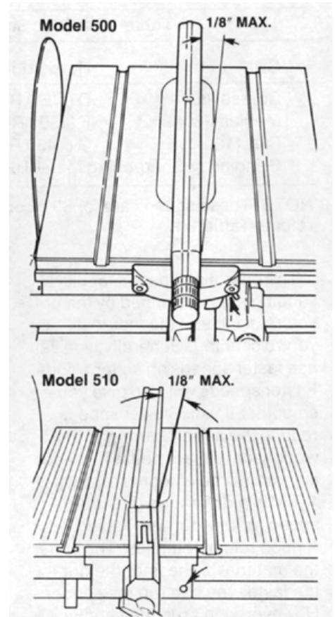
**Figure 17-7.** Offsetting the rip fence for endg sanding.
