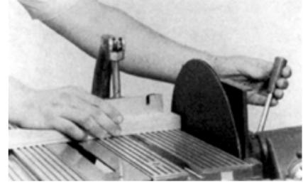
**Figure 17-4.** When using the quill feed, move the disc in and out as shown. Don't let the stock contact the abrasive for more than a few seconds at a time.
